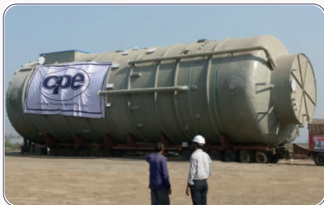
Largest FRP Equipment made in India. 10m ID x 35m height Scrubber. Project Location: Denmark
