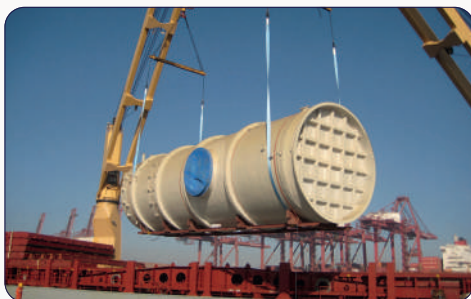
Cooling Tower for Copper Refinery 6.2m ID x 23m height. Project Location: Zambia
