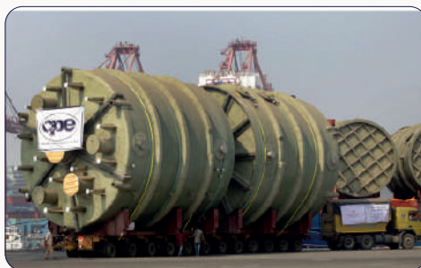
FRP Reactors. 8.5m ID x 9m height. Project Location: Singapore
